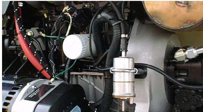
Lube Point(s) - Replaceable Element
