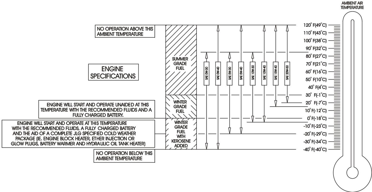
**Figure 6-2. Engine Operating Temperature Specifications - Deutz - Sheet 1 of 2**
