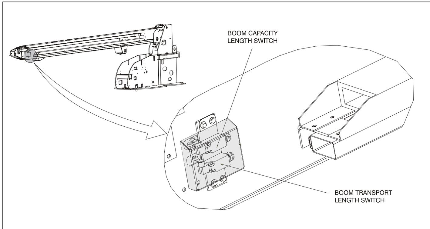
Figure 2-7. Limiting and Cut-Out Switches - Sheet 2 of 2
