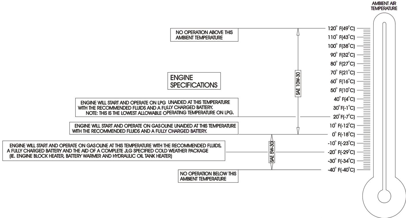
**Figure 6-8. Engine Operating Temperature Specifications - GM - Sheet 1 of 2**
