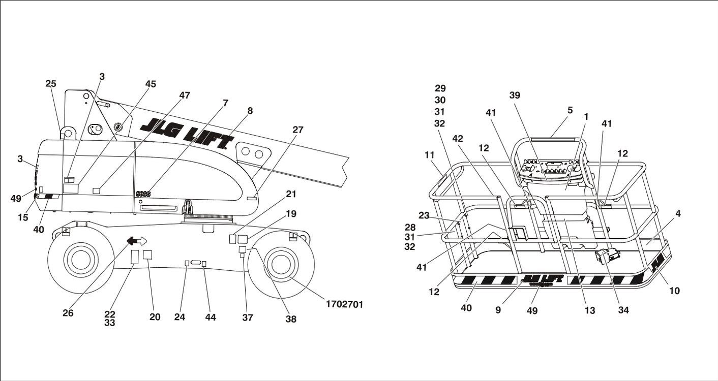
Figure 4-8. Decal Location - Rear Entry Platform - Sheet 2 of 2
