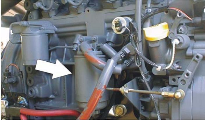
Lube Point(s) - Replaceable Element
