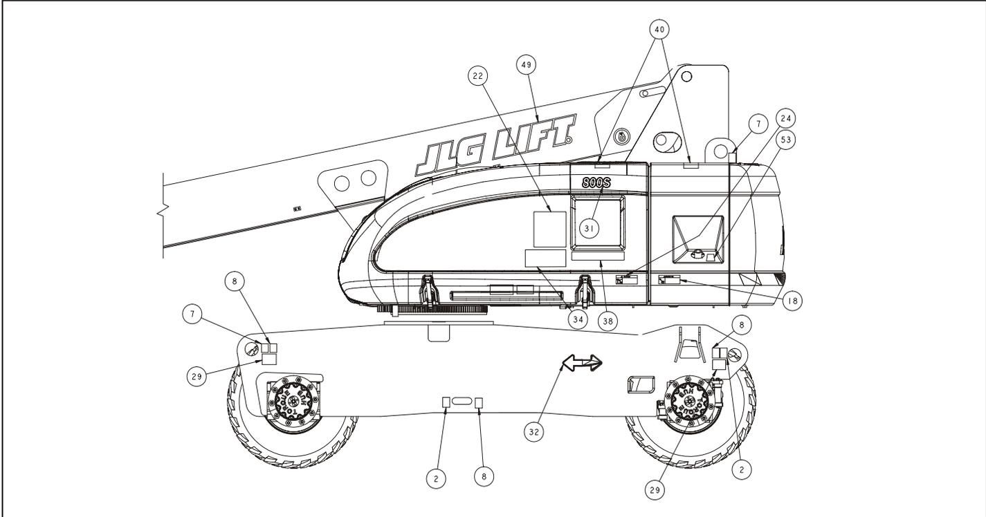
Figure 4-10. Decal Location - Side Entry Platform - Sheet 2 of 5
