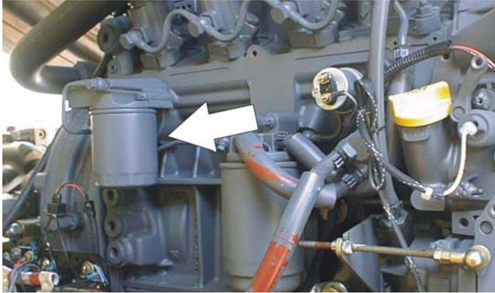
Lube Point(s) - Fill Cap/Spin-on Element (JLG P/N 7016331)
