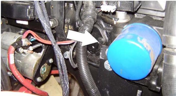
Lube Point(s) - Fill Cap/Spin-on Element
