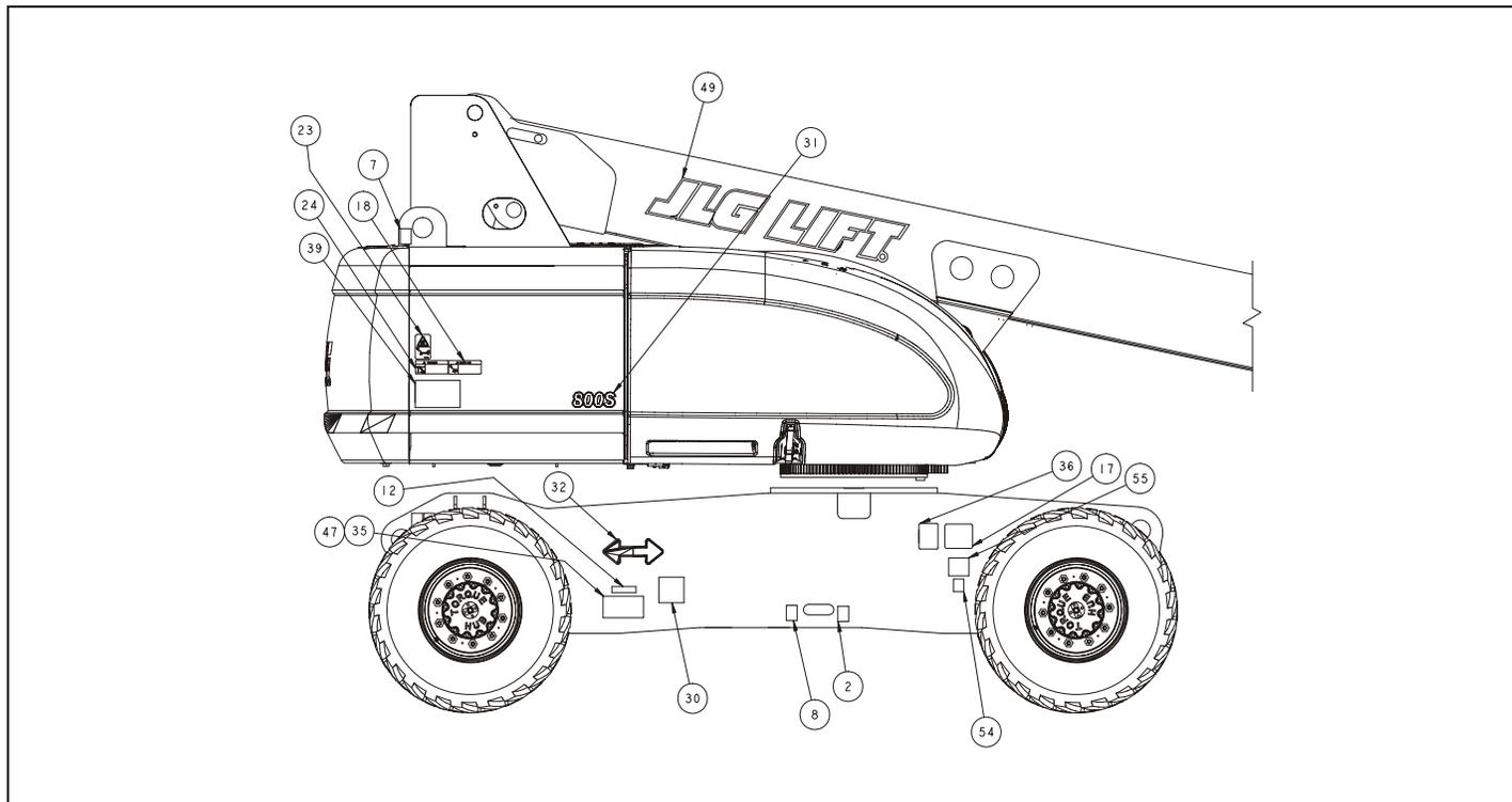
Figure 4-9. Decal Location - Side Entry Platform - Sheet 1 of 5
