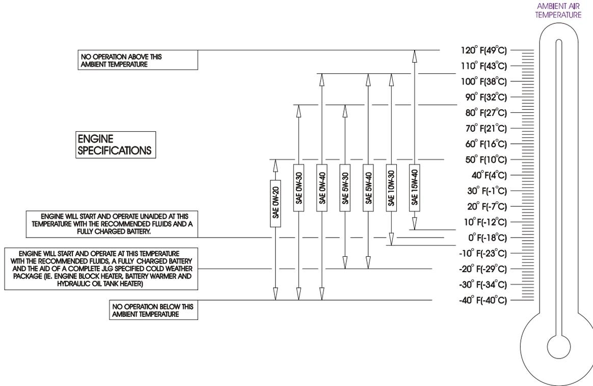
Figure 6-6. Engine Operating Temperature Specifications - Caterpillar - Sheet 1 of 2
