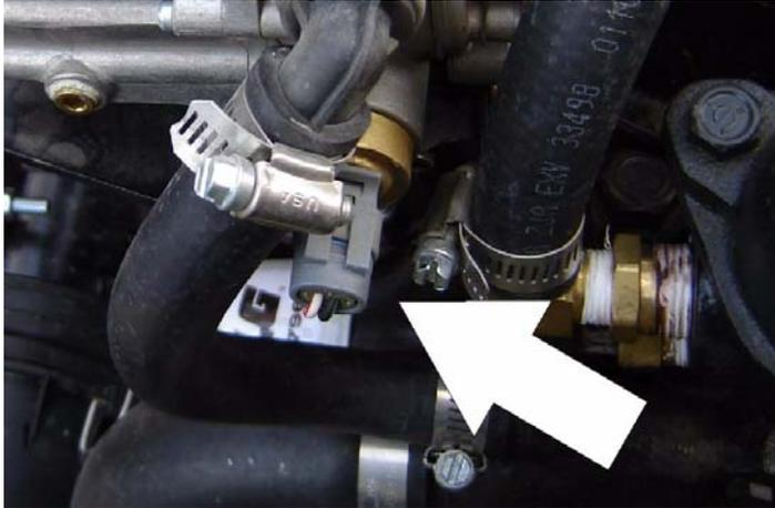
6. Remove the retainer clip for the LPG fuel temperature sensor and remove the sensor from the regulator body.
