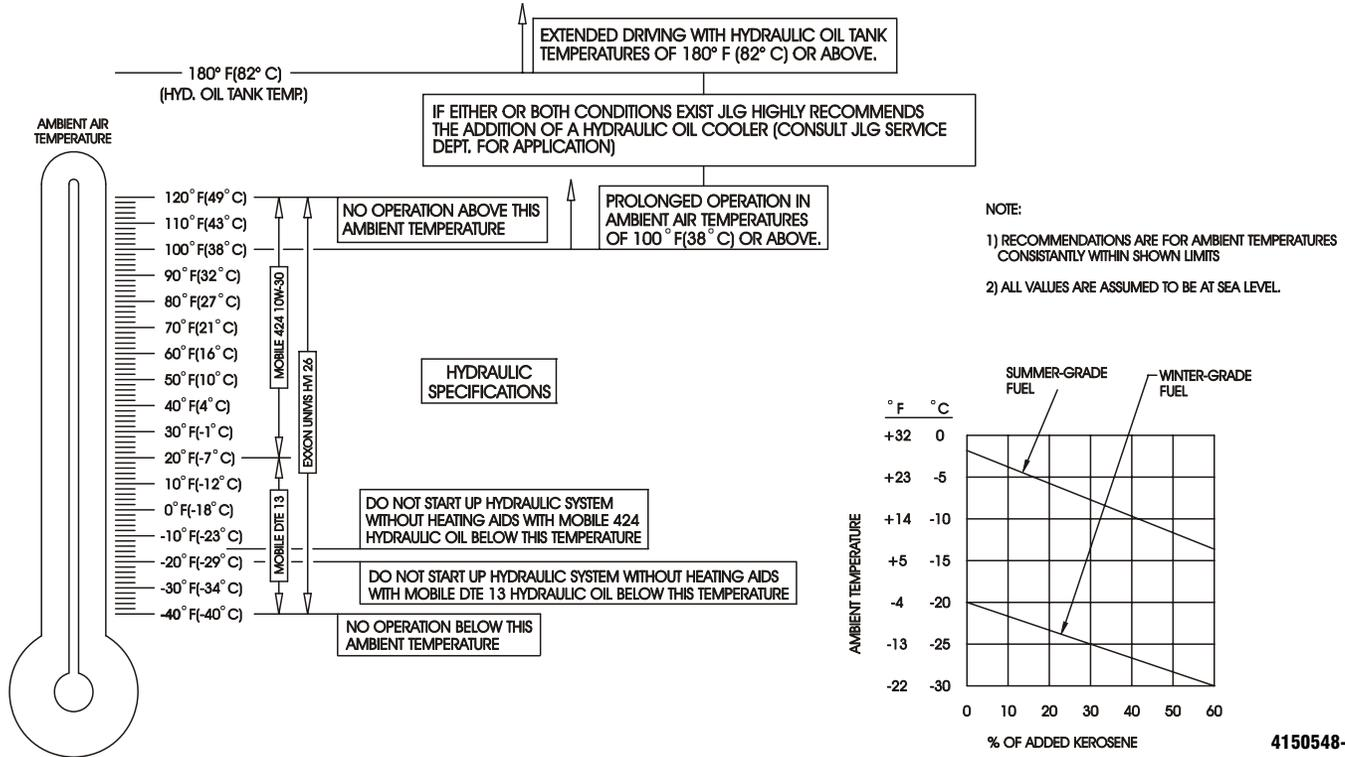
Figure 6-3. Engine Operating Temperature Specifications - Deutz - Sheet 2 of 2
