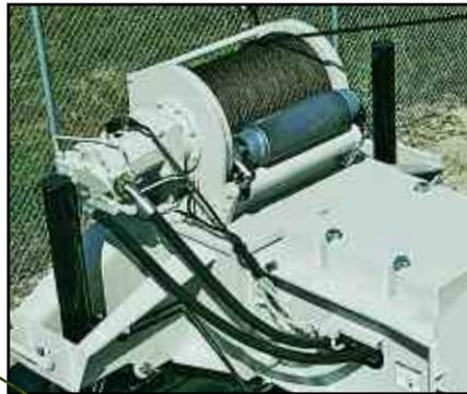
**Counterweight transfer removal controls** located on each side of the upper structure
