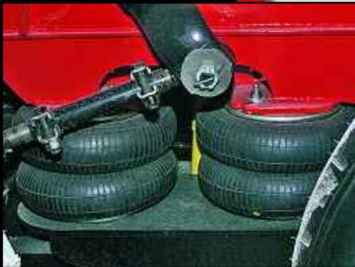
**Air-ride suspension** front and rear provides a smooth ride and precise handling. Optional air-ride lift system holds the rear suspension retracted while the crane is on outriggers.
