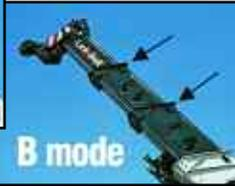
Exclusive **Amax mode** (mode "A") offers substantially increased capacities. **Standard mode** (mode "B") self-proportions all four sections equally.
