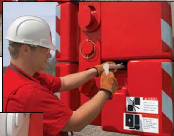
Simple lever action disengages counterweight pins from upper
