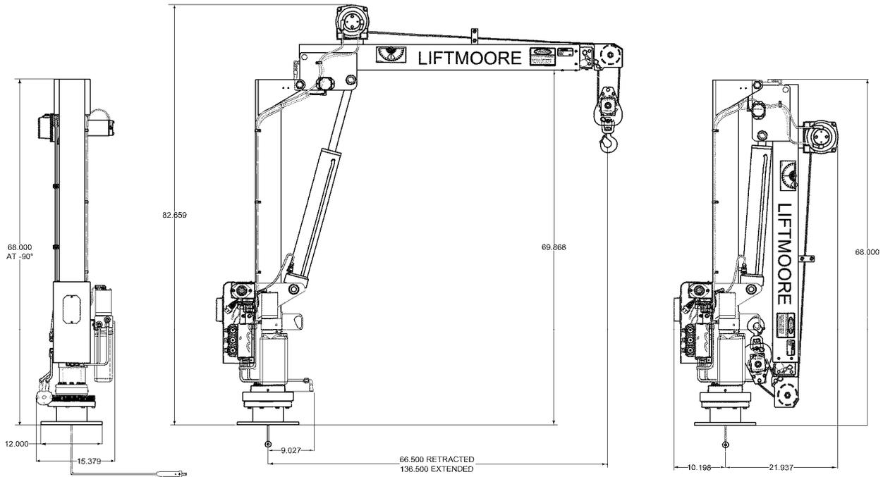
**HOIST WINCH:** The hoist winch uses a planetary gear drive for most efficient operation. The winch is powered by a permanent magnet electric motor. The single line capacity of the winch is 1200 Lbs. An integral mechanical brake is included with the winch.
